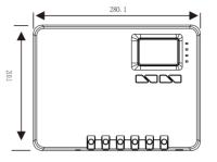
Product Size: 280.1\*210.1\*90.6mm Installation Size: 256\*154.5mm Installation Holes Diameter:φ2.5 & φ5 Connection Holes Size:7.5\*7.5mm
